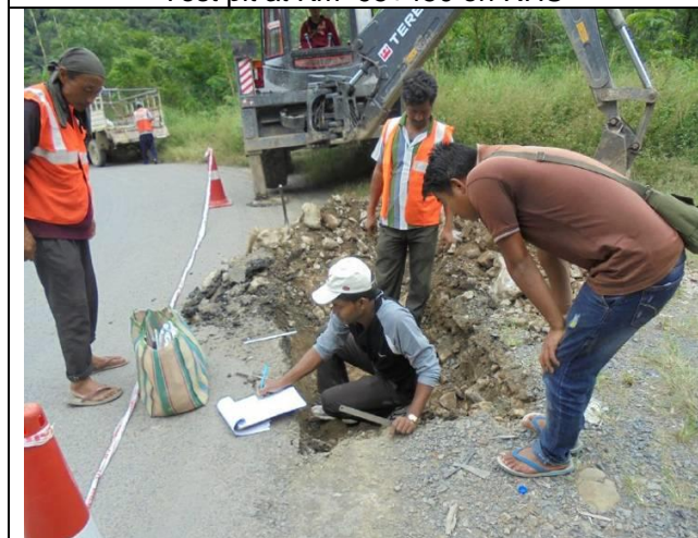
Measurement of existing crust composition at KM 101+600 on RHS
