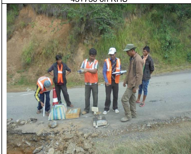
Field Dry Density Test at Km 54+140
