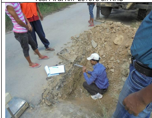
Measuring the existing crust composition at Km 43+730 on RHS
