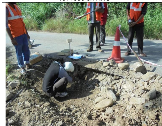
Measurement of crust composition at Km 107+500 on RHS
