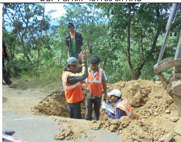
Test pit & DCPT at Km 48+825
