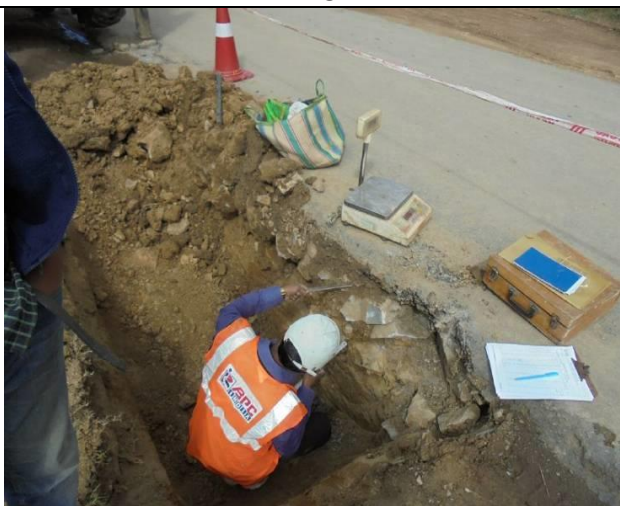
Measurement of existing crust at Km 63+150 on RHS
