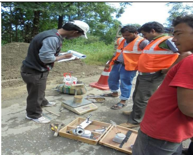
Measurement of Dry Density at Km 86+025 on LHS
